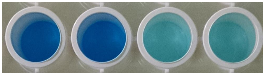
Figure 2. Left two wells contain qPCR reaction mix including Goof-Proof™ Master Mix and have had the DNA template or NTC control added in Template Buffer, hence the darker blue color. The right two wells have not yet had the DNA template or NTC control in Template Buffer added, and therefore are still the lighter blue of the 1X Goof-Proof™ Master Mix.
